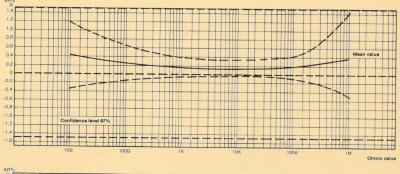
LOAD LIFE (W<sub>n</sub> for 1,000 hours at 70°C)
